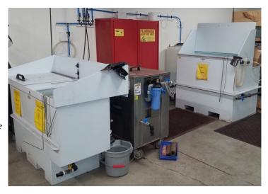
Right to Left: Benzyl Alcohol Lacquer Strip and Rinse, Ultrasonic Aqueous System, Rinse Tank
